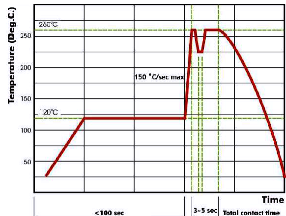
Recommended wave soldering profile for SMT process with SnAgCu series solder.
