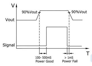
Figure 3. Power Good / Fail Signal Diagram
