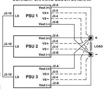
Figure 5. Current Sharing Block Diagram
