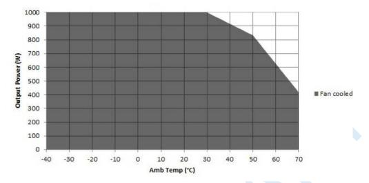
Figure 1. Power Derating Curve MBE1000
