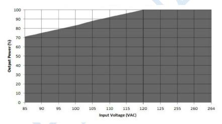
Figure 2. Power Derating Curve w.r.t. Input
