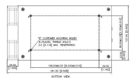
MECHANICAL OUTLINE DIMENSIONS ALL DIMENSIONS ARE IN MM [INCHES] GEN.TOLERANCE:±1.0 MM [±0.04]
