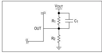
Figure 1. Adjustable Output-Voltage Configuration
