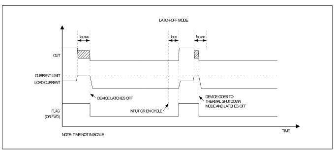
Figure 5. Latch-Off Fault-Timing Diagram
