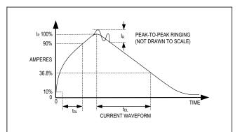
Figure 9. Human Body Current Waveform
