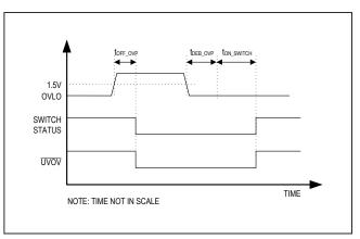
Figure 1. Overvoltage-Fault Timing Diagram
