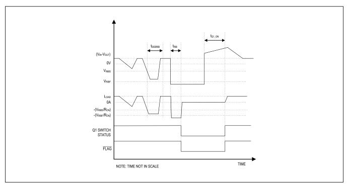
Figure 7. Fast Reverse-Current Fault-Timing Diagram
