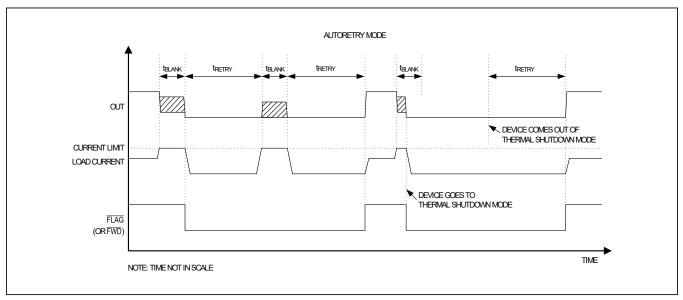
Figure 3. Autoretry Fault-Timing Diagram
