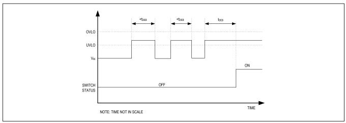
Figure 2. Debounce Timing Diagram
