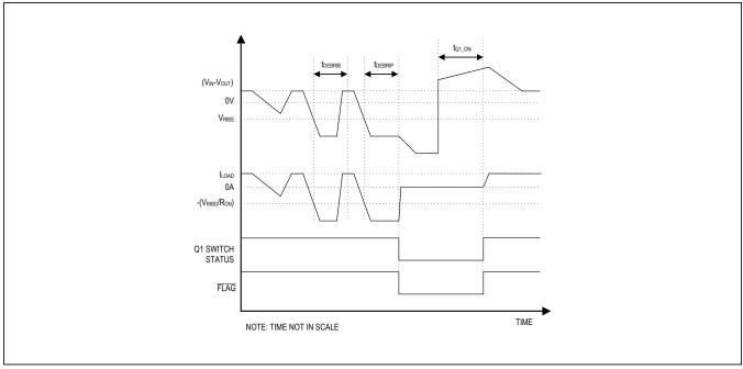
Figure 6. Slow Reverse-Current Fault-Timing Diagram
