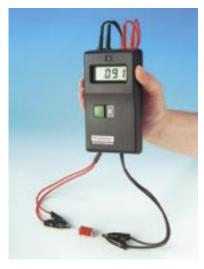
This instrument is a portable digital meter to measure low resistances over the range  $0.001\Omega$  to  $200\Omega$ . A high degree of accuracy is achieved by utilising a four terminal input to eliminate errors caused by test lead length.
