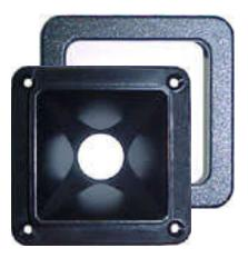
OPTION Q Square Bezel Snap-on Front mount (FM) Cutout = 1.25" [31.75mm] (Bezel covers screws)
