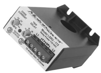
The Model LSRU load sensors use current levels to monitor all types of over and underload conditions such as feed rates, tool wear, pump loads, mixer viscosity and others. They may be used to stage pumps, chillers and other machinery. Two user adjustments are provided with your choice of overcurrent, undercurrent, trip delay, restart delay and extended restart delay options. Three current ranges, 0-10A, 5-25A and 25-100A, are available.
