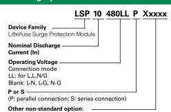
X3333: without GND wire connection, available for 240Vac and 277Vac rating with CE Marking for Class I unearthed installation. Wire Color: Line: Brown, Neutral: Blue, Ground/P: Green with yellow stripe
