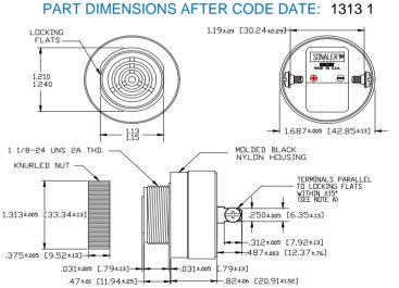
NOTE A: TERMINALS-.032 BRASS TIN PLATED, TAPPED FOR #6-32 SCREW, TWD #6-32 NICKEL PLATED BRASS SCREWS INCLUDED, WILL ACCEPT 1/4' QUICK CONNECT. NOTE B: MOUNTING- REMOVE BLACK PLASTIC NUT AND INSERT THREADED FRONT THREUGH 1.25' HOLE PUNCHED IN PANEL, IF DRIENTATION IS NEEDED, NOTE LOCKING FLATS ON DRAWING. SCREW NUT BACK ON. DO NOT OVERTIGHTEN.
