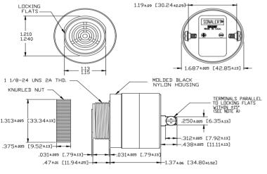
NOTE A: TERMINALS-.032 BRASS TIN PLATED, TAPPED FOR #6-32 SCREW. TVOI #6-32 NICKEL PLATED BRASS SCREWS INCLUDED. WILL ACCEPT 1/4' QUICK CINNECT.
