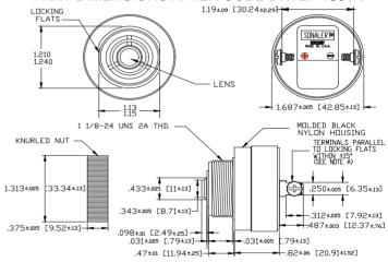
NOTE A: TERMINALS-.032 BRASS TIN PLATED, TAPPED FOR #6-32 SCREW, TWD #6-32 NICKEL PLATED BRASS SCREWS INCLUDED, WILL ACCEPT 1/4' QUICK CONNECT. NOTE B: MOUNTING- REMOVE BLACK PLASTIC NUT AND INSERT THREADED FRONT THROUGH 1.25° HOLE PUNCHED IN PANEL, IF DRIENTATION IS NEEDED, NOTE LOCKING FLATS ON DRAWING, SCREW NUT BACK ON. DO NOT OVERTIGHTEN.
