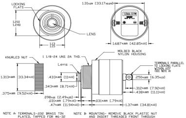
NOTE A TERMINALS-032 BRASS TIN PLATED, TAPPED FOR #6-32 SCREW, TWO 16-32 NICKEL PLATED BRASS SCREWS INCLUDED, WILL ACCEPT 1/4\* QUICK CONNECT. NOTE B: MOUNTING- REMOVE BLACK PLASTIC NUT
