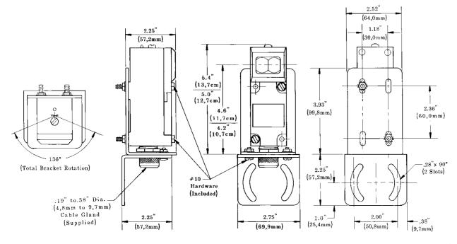
Figure 4. SMBLS Bracket Dimensions
