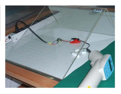
Note : the assembly has a heat shrinkable tube to cover & protect the entire secondary circuits to meet ESD and Hipot test requirement
