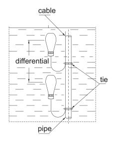
wiring diagram for emptying pump
