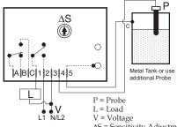
$\Delta S = Sensitivity Adjustment$ Connect common to conductive tank or an additional probe as required. Contacts A, B & C are isolated.
