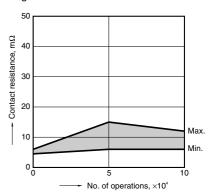
6-2. Electrical life test (UL lamp load test TV-5) Tested sample: LK1aF-12V, 6 pcs.
