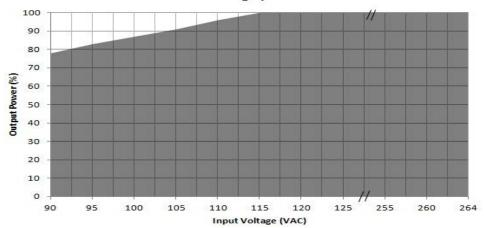
De-rate linearly from 100% at 115VAC to 78% at 90VAC
