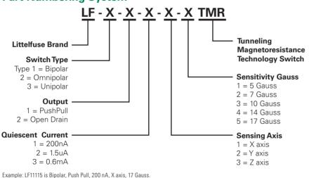
Example: LF11115 is Bipolar, Push Pull, 200 nA, X axis, 17 Gauss. Note: Every combination is NOT offered. Contact Littelfuse for availability.
