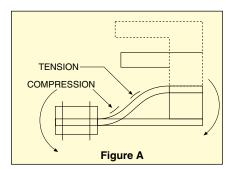
Two typical mounting arrangements are shown below. For high-accuracy applications, reinforcement plates should be slightly harder than the beam material, and the interfacing corners should be sharp. Because of low loads and sensor construction associated with the LCL113G through LCL-816G, in-line loading (Type 2) is not recommended.
