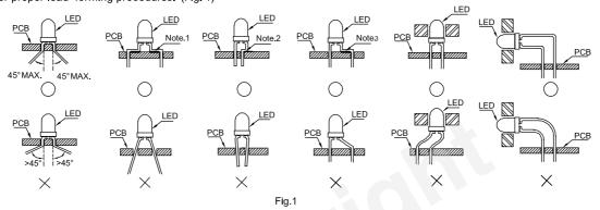
"Correct mounting method "X" Incorrect mounting method
