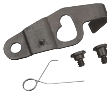
Short-stop Latch protects wire strands by limiting the stripping stroke to \frac{3}{32} in. and retains the slug until the wire is ready for terminating.
