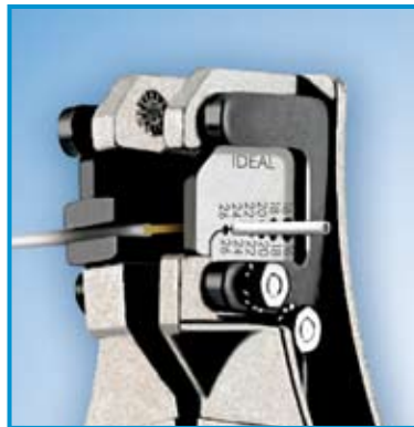
Die-type blades incorporate a counterbored hole sized to the insulation and an inner cutting hole sized to the conductor. This varies depending on insulation type and thickness.
