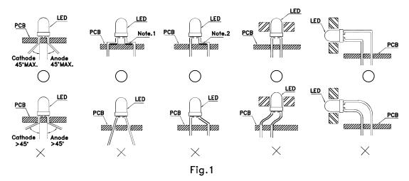
$"\bigcirc$  " Correct mounting method "imes" Incorrect mounting method
