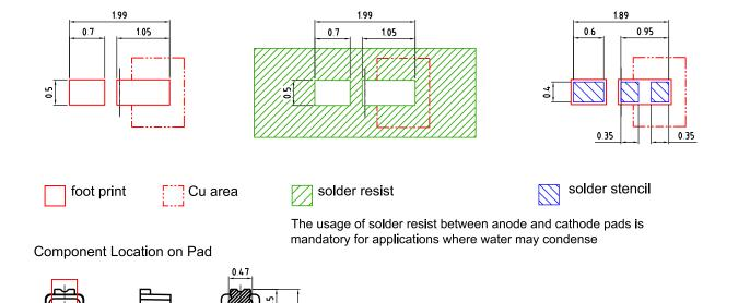
For superior solder joint connectivity results we recommend soldering under standard nitrogen atmosphere.
