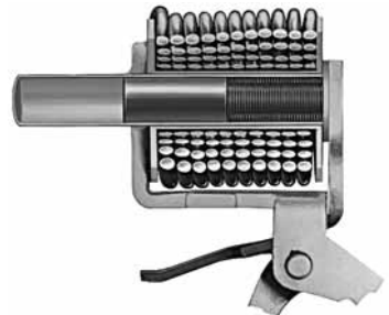
Armature Pulled In
