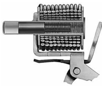
Overload Subsides Before Core Reaches Pole Piece
