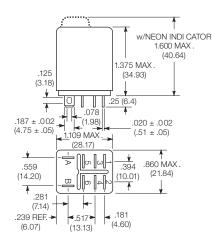
Mounting code 5 Printed circuit terminals
