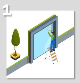
Install SafeCount sensors above entrance and connect cables
