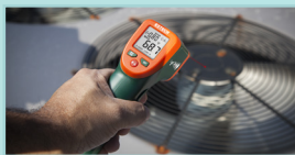
Test for temperature in HVAC systems
