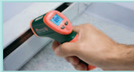
Test for temperature in heating systems
