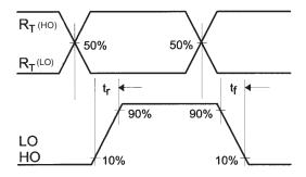
Figure 2. Switching Time Waveform Definitions
