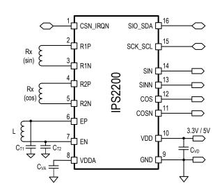
Configuration with split capacitors CT1 and CT2 for improved EMC performance. Both capacitors must have the same capacitance.
