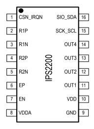
Figure 1. Pin Assignments for 4.4mm × 5.0mm 16-TSSOP Package - Top View
