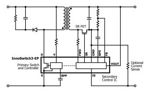
Figure 1. Typical Application Schematic.
