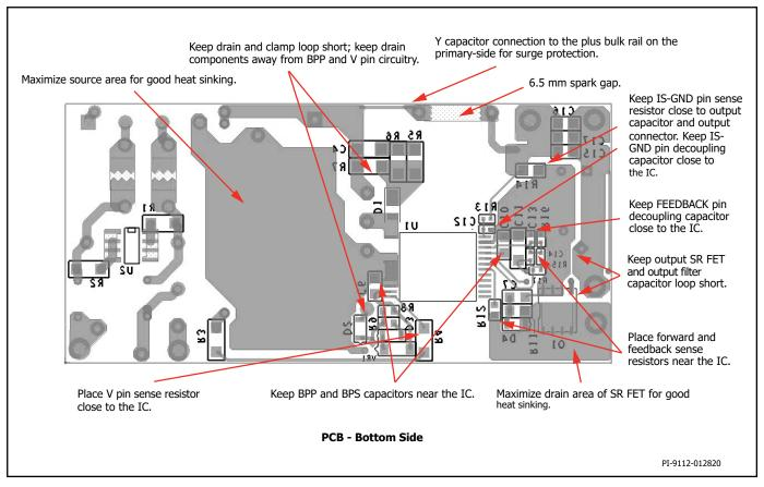
Figure 12. PCB Layout.
