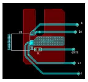
Figure 23. Ther3mal Resistance Test Conditions for PowiGaN Devices (INN3678C, INN3679C and INN3670C.)
