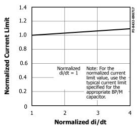
Figure 29. Standard Current Limit vs. di/dt.
