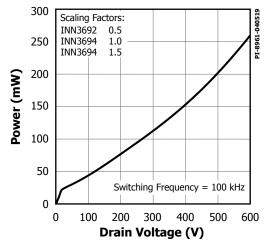
Figure 33. Drain Capacitance Power.
