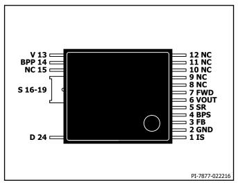
Figure 5. Pin Configuration.
