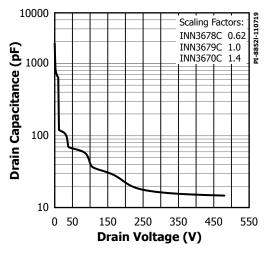
Figure 36.  $C_{\rm oss}$  vs. Drain Voltage.
