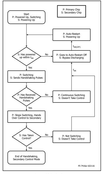
Figure 7. Primary-Secondary Handshake Flowchart.
