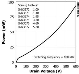
Figure 27. Drain Capacitance Power.
