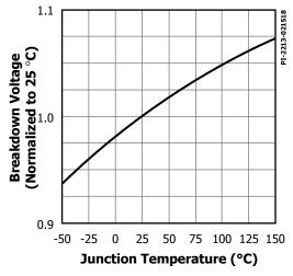
Figure 34. Breakdown vs. Temperature (Exclude INN3678C / INN3679C / INN3670C).
