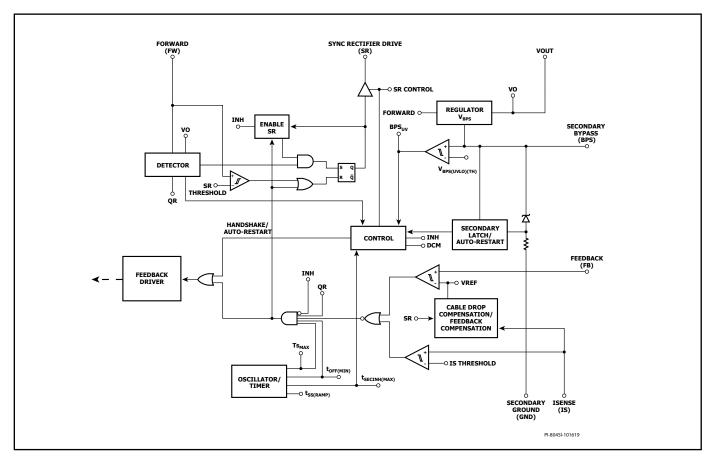
Figure 4. Secondary Controller Block Diagram.
