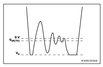
Figure 13. Unacceptable FORWARD Pin Waveform After Handshake with SR Switch Conduction During Flyback Cycle.
