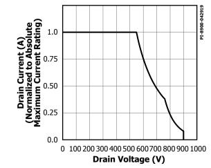
Figure 30. Maximum Allowable Drain Current vs. Drain Voltage (INN369x).
