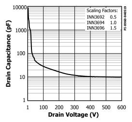
Figure 32.  $C_{oss}$  vs. Drain Voltage.
