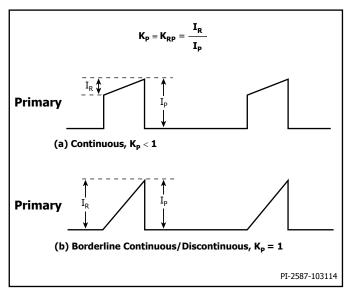
Figure 20. Continuous Conduction Mode Current Waveform, KP < 1.
