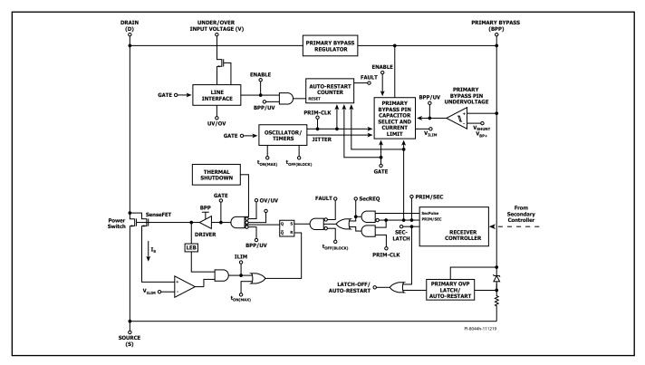
Figure 3. Primary Controller Block Diagram.
