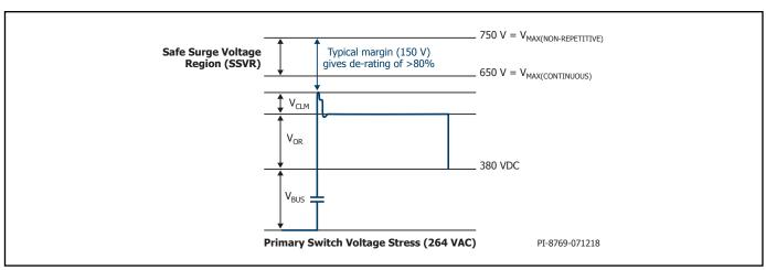
Figure 22. Peak Drain Voltage for 264 VAC Input Voltage.
