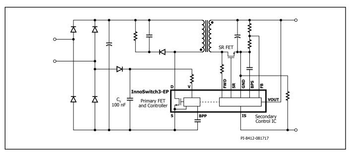
Figure 18. Fast AC Reset Configuration.
