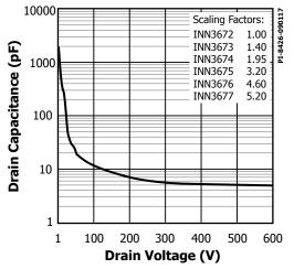
Figure 26.  $C_{\rm oss}$  vs. Drain Voltage.
