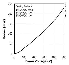
Figure 37. Drain Capacitance Power.
