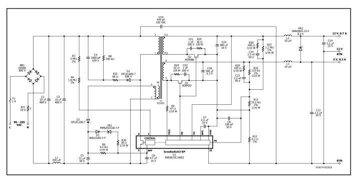
Figure 10. Schematic DER-611, 5 V, 0.3 A and 12 V, 0.7 A for HVAC (Heating, Ventilation and Air-Conditioning) Application.
