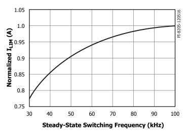
Figure 6. Normalized Primary Current vs. Frequency.
