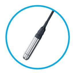
The ILTSU is designed for use in continuous submersion in liquids such as water, oil and fuels. The probe uses the latest piezo-resistive media-isolated silicon sensing technology and a stainless steel diaphragm. Housed within a 316L stainless steel, or high grade Duplex stainless steel housing, this submersible transmitter is the ideal product for hydrostatic level measurement where temperature is also a critical part of the measurement.
