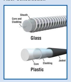
**Core**-Thin glass or plastic center of the fiber through which light travels.
