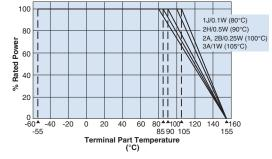
For resistors operated at a terminal part temperature of described for each size or above, a power rating shall be derated in accordance with the above derating curve. Please refer to "Introduction of the derating curve based on the terminal part temperature" in the beginning of our catalog before use.
