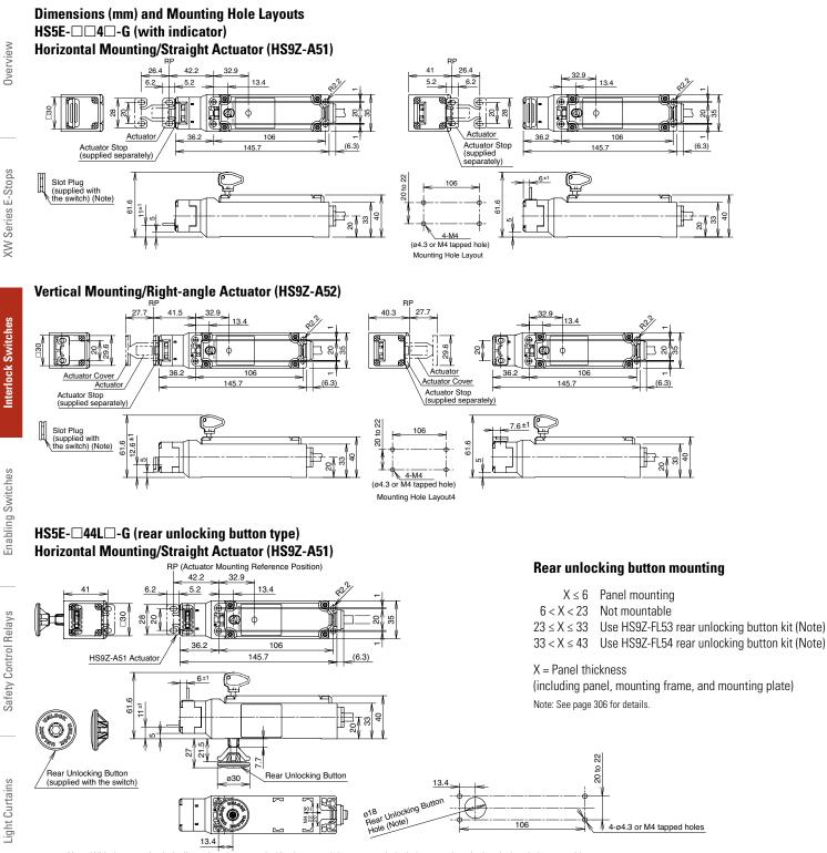
Note: With the mounting hole dimension, the rear unlocking button rod does not touch the hole even when the interlock switch moves sideways.
