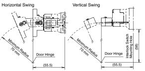
When the door hinge is on the extension line of the actuator mounting surface: 70 mm
