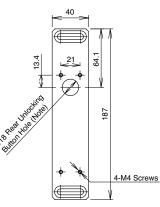
**Drilling Rear Unlocking Button Hole**
