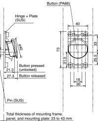
Rear Unlocking Button Kit Mounting Hole Layout
