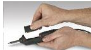
Collection chamber replacement
