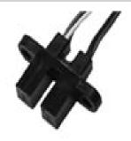
HOA Series IR Opaque Optoschmitt Sensor, Transistor Output, Two Mounting Tabs, Plastic Package
