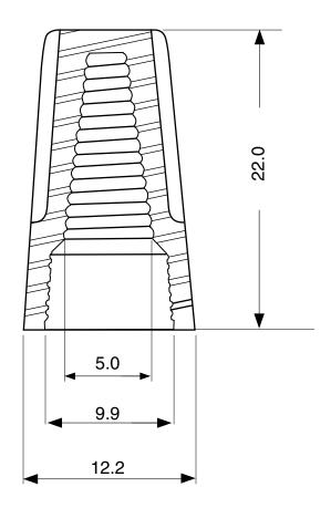
Working Temperature: 105° C Wire Range: #22 - #14 AWG
