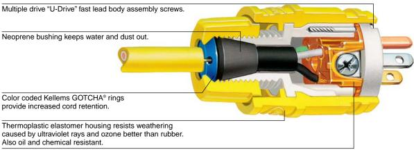
Three separate transparent wiring chambers allow for visual inspection.
