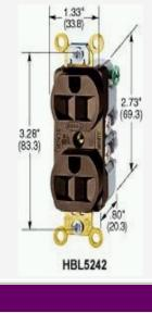
2-Pole 3-Wire Grounding, 15A 125V, 5-15R, Flush Nylon Face, Side Wired Only, Brown
