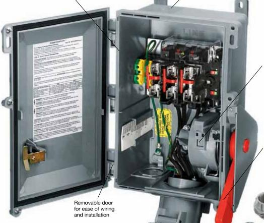
The patented Plug-Check™ mechanism detects the presence of the plug. It operates as a clutch to engage the handle with the switch and captures the plug. This action prevents the plug from being removed until the switch is turned OFF
