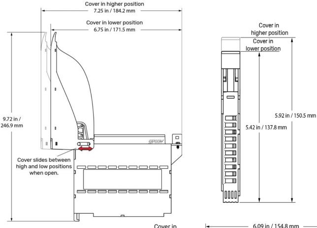
The module cover pivots and can be adjusted to two different heights (positions). The higher position provides more space to accommodate thicker wires.
