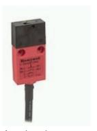
GKM Series, Miniature Key Operated Safety Interlock Switch, 1NC/1NO Direct Opening, Slow Action, 3 m Bottom Exit Cable, Plastic Housing, Silver Contacts
