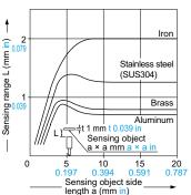
As the sensing object size becomes smaller than the standard size (iron sheet  $10 \times 10 \times t$  1 mm  $0.394 \times 0.394 \times t$  0.039 in), the sensing range shortens as shown in the left figure.
