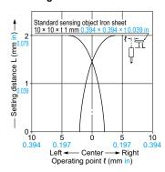
The graph on the left is plotted with the sensitivity adjusted so as to just detect a  $10 \times 10 \times t$  1 mm  $0.394 \times 0.394 \times t$  0.039 in iron sheet placed at a distance of 2.0 mm 0.079 in.
