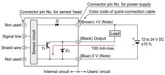
Note: The quick-connection sub cable does not have +V (brown) and 0 V (blue). The power is supplied from the connector of the main cable.
