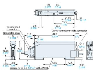
Note: The front view shows the sensor head connector and quick-connection cable connector attached.
