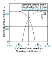
The graph on the left is plotted with the sensitivity adjusted so as to just detect a  $5 \times 5 \times t$  1 mm  $0.197 \times 0.197 \times t$  0.039 in iron sheet placed at a distance of 1.0 mm 0.039 in.
