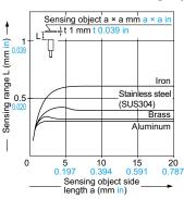
As the sensing object size becomes smaller than the standard size (iron sheet  $5 \times 5 \times t$  1 mm  $0.197 \times 0.197 \times t$  0.039 in), the sensing range shortens as shown in the left figure.
