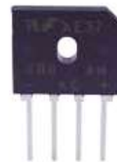
Rectifier for AC supply
