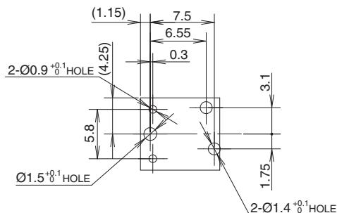
\*Please study & choose other appropriate hole diameters if confirmed the diameter values recommended above don't work with the soldering process.
