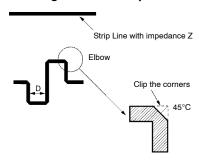
When the lines must curve, an elbow can be used as shown in the diagram. A distance (D) between the lines of approximately twice the line width is sufficient.
