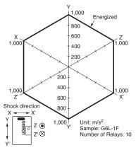
Conditions: Shock is applied in ±X, ±Y, and ±Z directions three times each with and without energizing the Relays to check the number of contact malfunctions.
