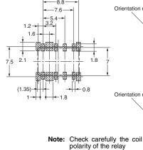
Terminal Arrangement and Internal Connections (Top View)
