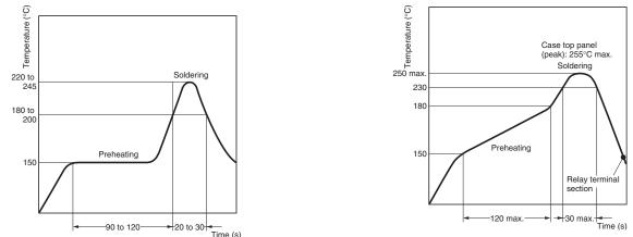
3. The thickness of cream solder to be applied should be between 200 and 250 μm and the land pattern should be based on Omron's recommended PCB pattern. To maintain the correct soldering joint shown in the following diagram, we recommend applying solder using the soldering conditions shown above. Check the soldering in the actual mounting conditions prior to use.
