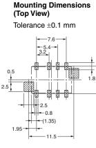
Note: Check carefully the coil polarity of the relay
