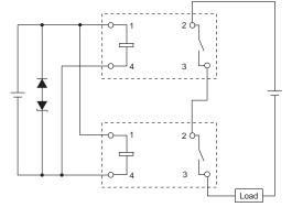
Note. The diode and zener diode are for the absorption of coil surge. (The coil does not have a polarity.) The opening/closing part does not have a polarity.
