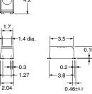
Note: A tolerance of  $\pm 0.1$  mm applies to all dimensions unless otherwise specified.
